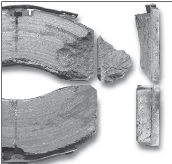
FIGURE 21: MAJOR BREAKOUTS ON THE SURFACE OF THE BRAKE PAD ARE NOT PERMITTED
