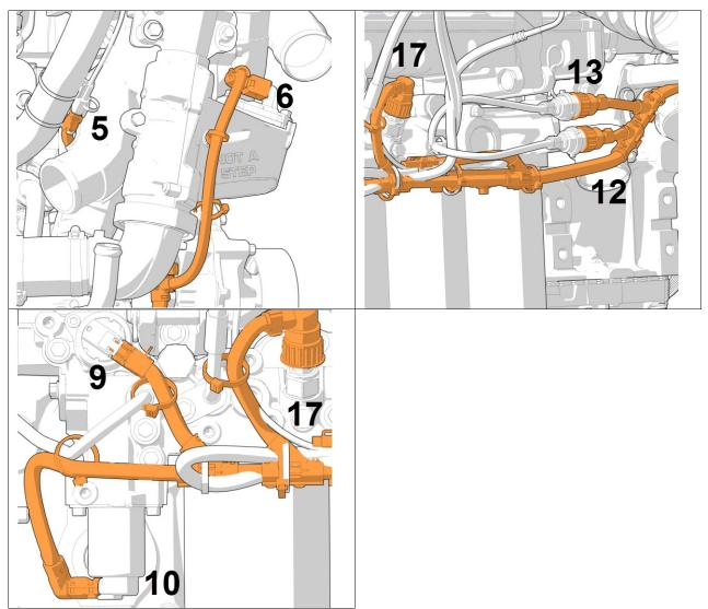
FIGURE 2: ENGINE HARNESS CONNECTION POINTS
