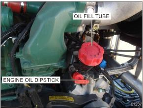
FIGURE 12: TYPICAL ENGINE OIL FILLING TUBE
