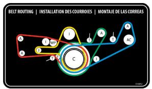
FIGURE 20: VIP BELT ROUTING - SMALL A/C SYSTEM,
