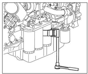
FIGURE 10: OIL FILTER WRENCH
