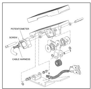
FIGURE 18: ELECTRONIC FOOT PEDAL ASSEMBLY 3035
