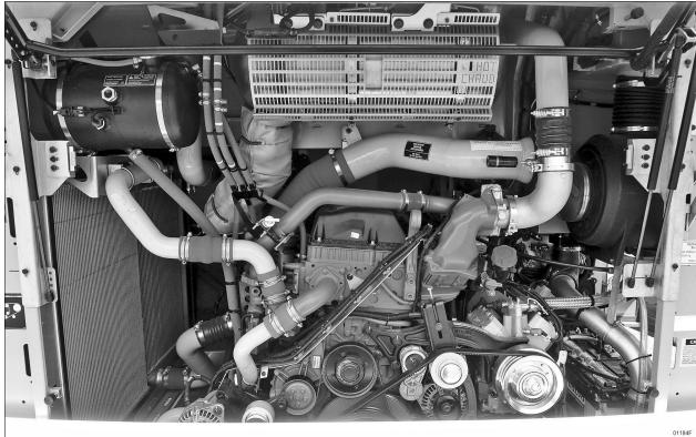
FIGURE 16: TYPICAL X SERIES ENGINE COMPARTMENT
