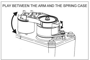
FIGURE 26: CHECKING BUSHING WEAR
