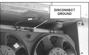
FIGURE 32: COOLING ASSEMBLY GROUND
