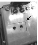
8. Slightly lift the door with the lift table to disengage the lower hinge pin and allow shroud removal from the vehicle.
