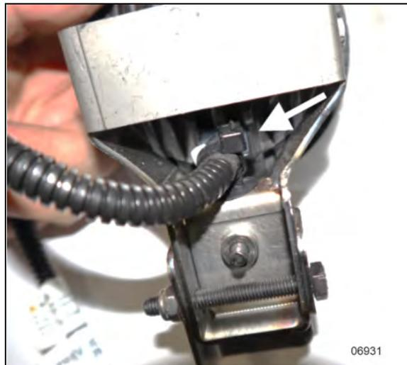
**FIGURE 108: FOG LIGHT INSTALLATION**
