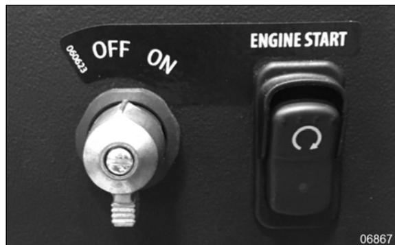
FIGURE 61: SWITCH ARRANGEMENT WITH STARTING MODULE
