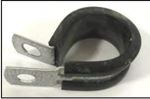
Figure 21: P-clamps are no longer used to secure power cables, but they can nevertheless be found on coaches of older generations. The piece of rubber that protects cable against the P-clamp steel loop must absolutely be in place. Replace any P-clamps where the rubber piece is missing, broken or likely to separate from the steel loop.
