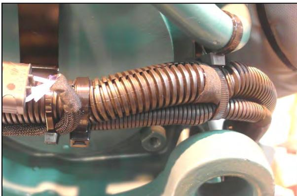
Figure 13: starter cables in a corrugated protective sheath.
