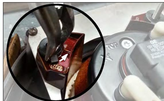
FIGURE 79: LOCK THREADED ROD
