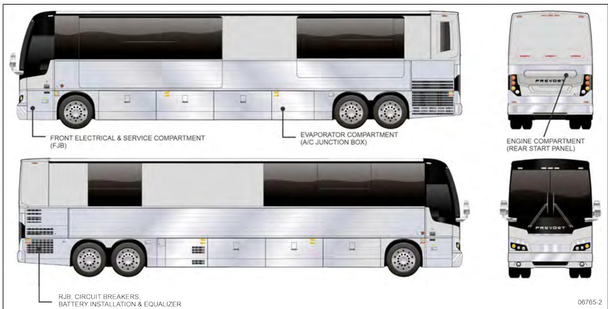
FIGURE 15: ELECTRICAL COMPARTMENTS (X3-45 VIP)
