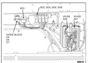
FIGURE 34: ENTRANCE DOOR & WIPER CONTROL PANEL
