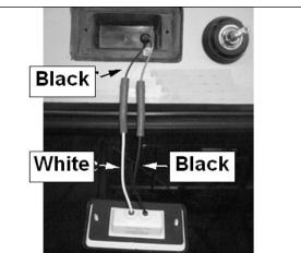
FIGURE 102: LED SEALED UNIT WIRE CONNECTION
