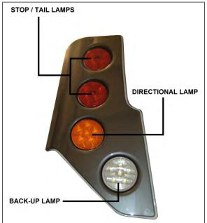
FIGURE 99: X3-SERIES REAR TAIL LAMPS, SOME VEHICLES MAY HAVE THE DIRECTIONAL LAMP MAY BE MOUNTED ON TOP POSITION
