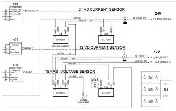
FIGURE 39: BATTERY CONNECTIONS SCHEMATIC - H3 SERIES
