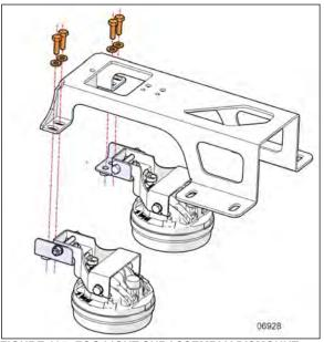
FIGURE 105: FOG LIGHT SUBASSEMBLY DISMOUNT
