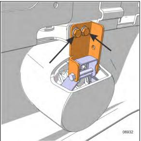
FIGURE 109: FOG LIGHT MOUNTING BOLT
