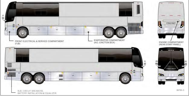
FIGURE 16: ELECTRICAL COMPARTMENTS (X3-45 VIP COMMERCIAL BUS SHELL)
