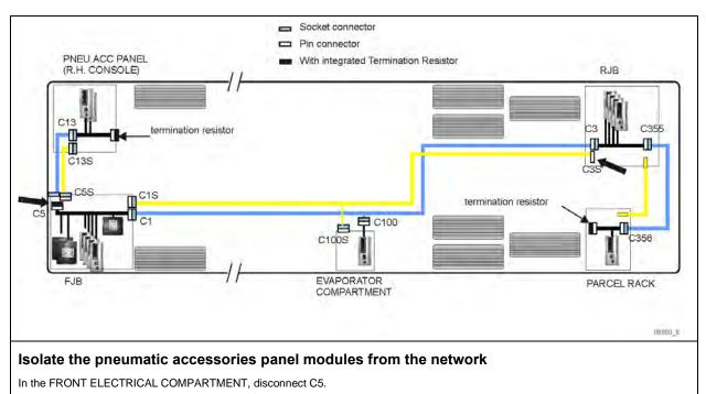
Take the spare termination resistor on C3S in the MAIN POWER COMPARTMENT and connect it to C5 pin housing.
