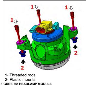
3. Using pliers, unfasten all plastic mounts from the headlight metal support (Figure 77).
