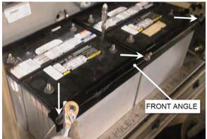
FIGURE 47: REMOVE THE FRONT ANGLE
