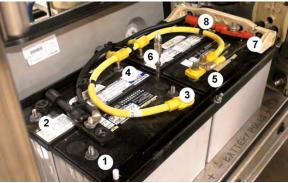
FIGURE 45: DISCONNECT 8 CABLE TERMINALS
