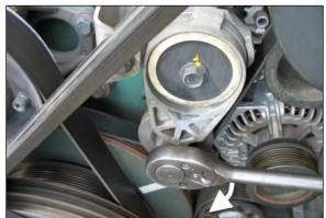
FIGURE 65: 1/2" SOCKET DRIVE WRENCH
