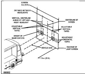
FIGURE 94: ALIGNMENT OF HEADLAMP AIMING SCREEN
