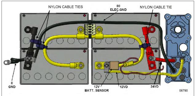
FIGURE 38: AGM BATTERY CONNECTIONS – X3 SERIES
