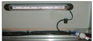
FIGURE 112: BAGGAGE COMPARTMENT LIGHTS LED SEALED UNIT
