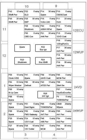
FIGURE 29: VECF – FUSE IDENTIFICATION
