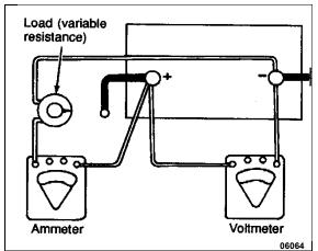
FIGURE 56: LOAD TEST
