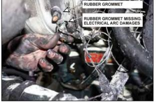
Figure 25: Fire in engine compartment caused by rubbing of power cable against metal edge of Bosch T1 alternator rear cover. Lower rubber grommet was missing when fire occured. Evidence of electrical arc can be seen.
