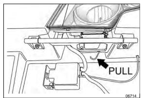
FIGURE 90: ROCKING THE HEADLAMPS ASSEMBLY
