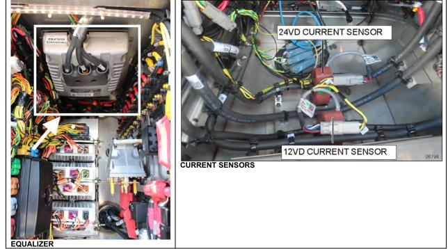
FIGURE 62: PRIME ELECTRICAL COMPONENTS
