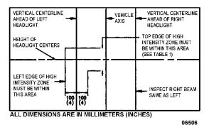
FIGURE 98: AIM INSPECTION LIMITS FOR LOWER-**BEAM HEADLAMPS**
