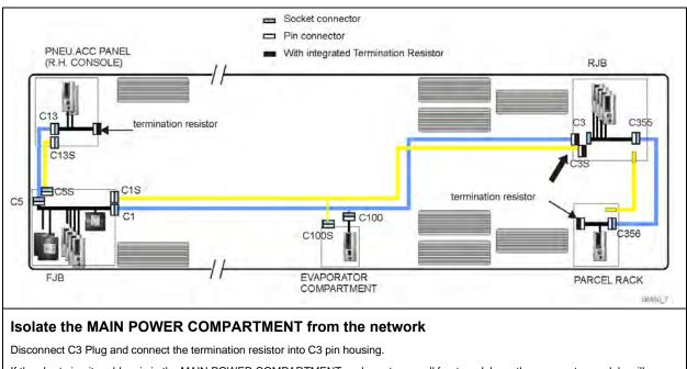
If the short circuit problem is in the MAIN POWER COMPARTMENT or downstream, all front modules + the evaporator module will respond normally.
