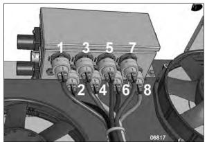
FIGURE 6: COOLING FANS CIRCUIT BREAKER BOX -CONNECTOR NUMBER
