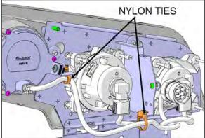
FIGURE 71: TYPICAL CABLE ROUTING WITH TWO HALOGEN HEADLAMPS
