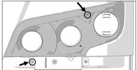
FIGURE 73: HEADLAMPS ASSEMBLY FIXING SCREWS
