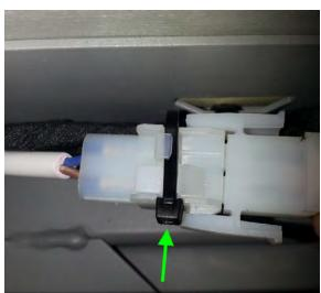
FIGURE 113: SECURE THE CONNECTOR WITH A NYLON TIE
