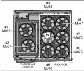
FIGURE 7: COOLING FAN IDENTIFICATION
