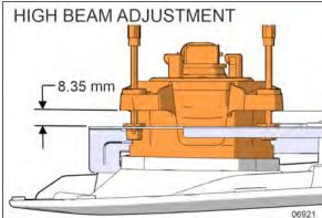
FIGURE 82: HIGH BEAM ADJUSTMENT
