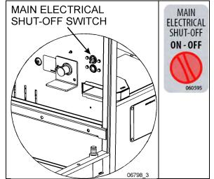
FIGURE 42: H3 SERIES MAIN ELECTRICAL SHUT-OFF SWITCH
