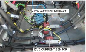
FIGURE 20: 12VD / 24VD CURRENT SENSORS IN MPC
