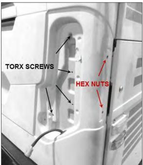
FIGURE 100: TAILLAMP POD RETAINING SCREWS & NUTS
