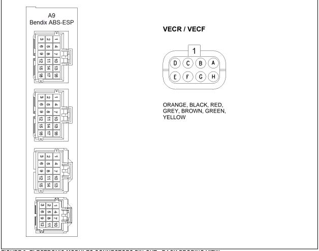
FIGURE 9: ELECTRONIC MODULES CONNECTORS PIN-OUT - BACK PROBING VIEW
