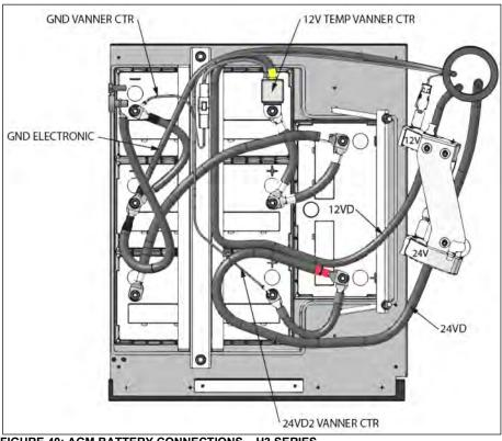
FIGURE 40: AGM BATTERY CONNECTIONS - H3 SERIES
