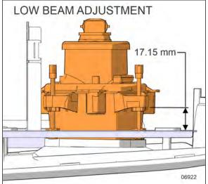
FIGURE 83: LOW BEAM ADJUSTMENT
