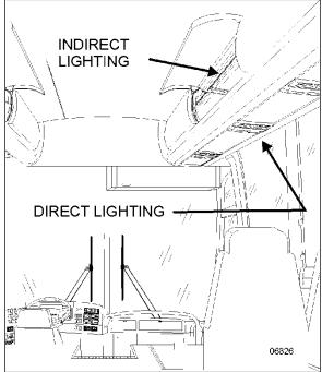
FIGURE 119: OVERHEAD COMPARTMENT LIGHTING
