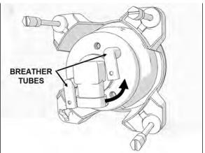
FIGURE 75: HALOGEN BULB REMOVAL
