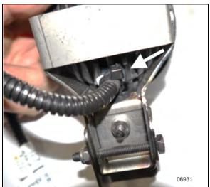
FIGURE 108: FOG LIGHT INSTALLATION
