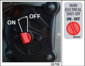
FIGURE 41: X3 SERIES MAIN ELECTRICAL SHUT-OFF SWITCH
