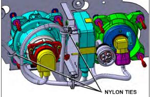
FIGURE 72: TYPICAL CABLE ROUTING WITH ONE XENON HEADLAMP (LEFT) AND ONE HALOGEN HEADLAMP (RIGHT). ROUTE THE XENON CABLE AROUND THE XENON HEADLAMP MODULE TO PREVENT ANY RISK OF FRICTIONAL WEAR
