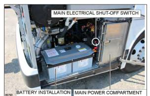
FIGURE 18: ENGINE R.H. SIDE COMPARTMENT
