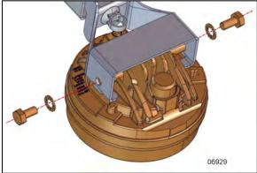
FIGURE 106: FOG LIGHT REMOVAL
