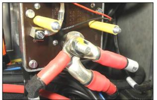
Figure 18: When several terminals are connected on a single stud terminal, the largest cable lug must be placed first, followed by the second larger and so on. Cable lugs should be distributed around the stud terminal in a way that no cable lug is distorted when tightening the nut.
