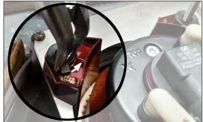
FIGURE 79: LOCK THREADED ROD
