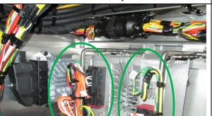
Disconnect the control connector from the battery equalizer (Optional)
