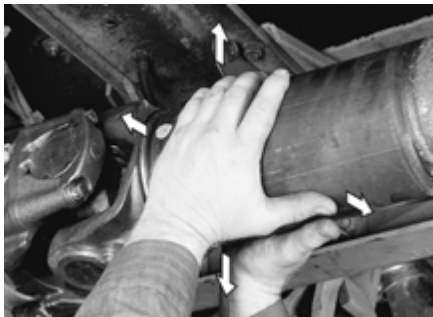
FIGURE 6: CHECK FOR LOOSENESS
