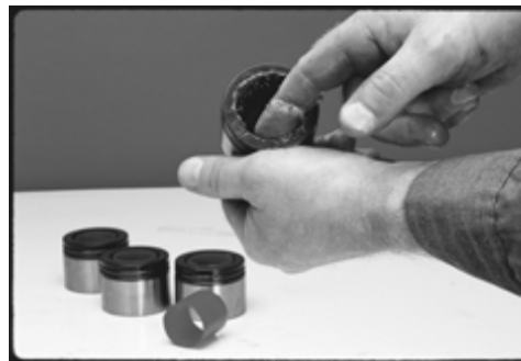
FIGURE 27: GREASING BEARING CUP
