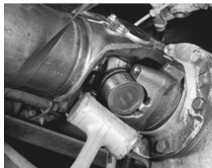
FIGURE 13: UNSEATING BEARING CUP ASSEMBLIES
