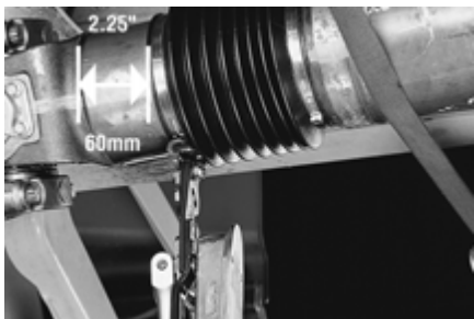
FIGURE 24: POSITION THE END OF THE BOOT AT THE 2.25 INCHES (55-60MM) MARK MADE ON THE YOKE SHAFT SHOULDER
