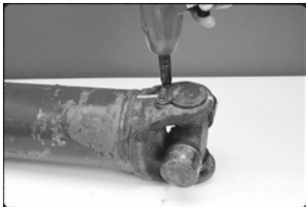
FIGURE 15: SPRING TAB BOLTS REMOVAL
