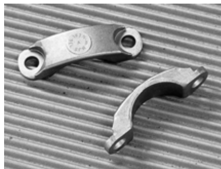
FIGURE 12: COLD FORMED BEARING RETAINERS
