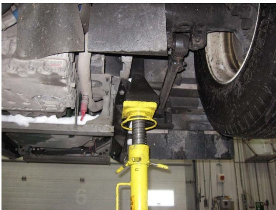
FIGURE 19 : JACK STAND AT CHASSIS HOISTING RECEPTACLE - AFT OF TAG AXLE, ROAD SIDE
