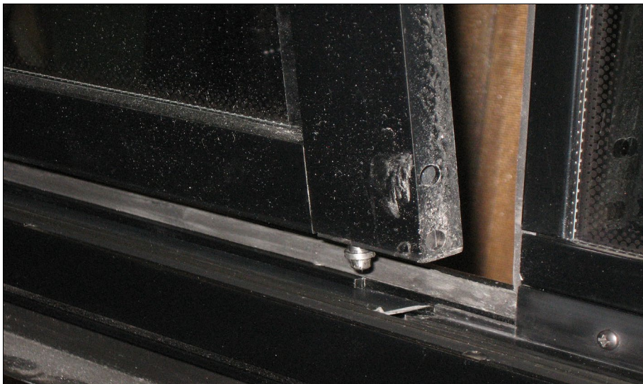
FIGURE 108: DISENGAGING THE BOTTOM OF THE SASH
