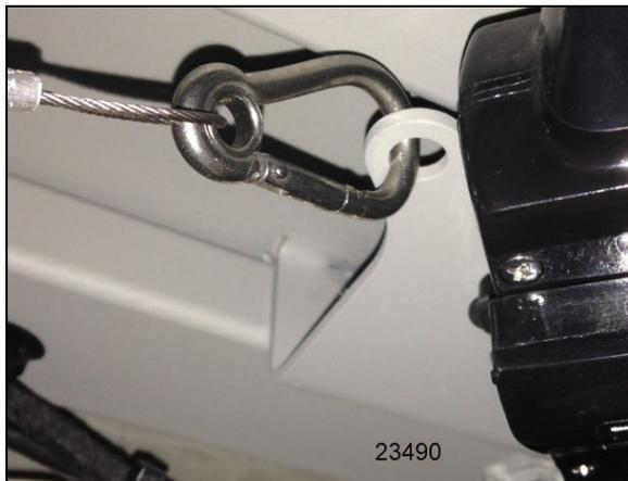
FIGURE 58: PROTECTIVE WIRE INSTALLATION
