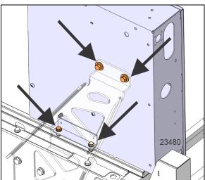
FIGURE 59: CONTROL BOX DISMOUNTING
