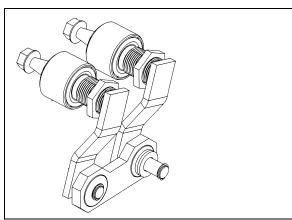
FIGURE 40: DRIVING MECHANISM (DRIVER SIDE) 23284
