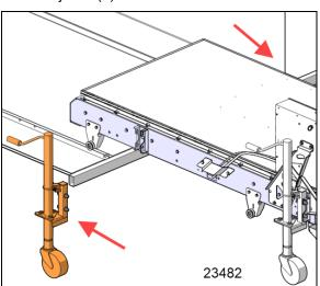
FIGURE 50: JACKS REMOVAL ON REAR SIDE
