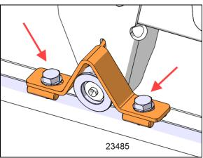
FIGURE 53: ANCHOR BOLTS INSTALLATION
