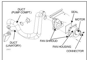
FIGURE 25: VENTILATION FAN INSTALLATION
