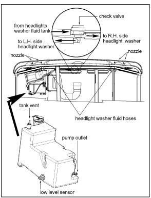
FIGURE 32: HEADLIGHTS CLEANING SYSTEM
