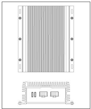
FIGURE 8: MULTICHANNEL POWER AMPLIFIER
