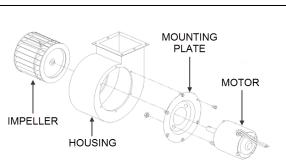
FIGURE 26: FAN ASSEMBLY COMPONENTS
