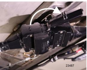
FIGURE 57: ELECTRICAL DISCONNECTION
