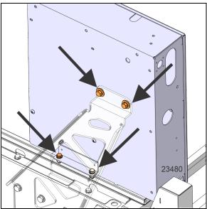
FIGURE 54: CONTROL BOX DISMOUNTING
