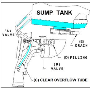
FIGURE 29: SUMP TANK SERVICE VALVES
