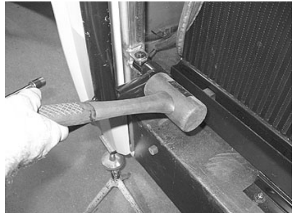
FIGURE 64: PANTOGRAPH ARM ADJUSTMENT
