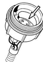
8. Apply clean engine oil to the water separation bowl new gasket. **Do not install pre-GHG17 fuel filters on GHG17 engines.**
