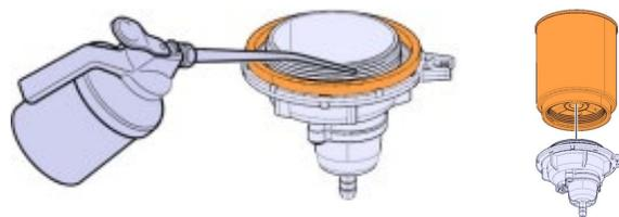
9. Install the new filter to the bowl. Tighten the filter by hand. Do not overtighten.
