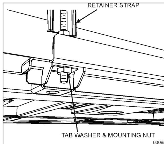
FIGURE 23: FUEL TANK STRAP MOUNTING
