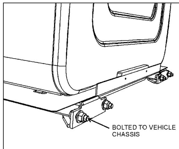
FIGURE 22: FUEL TANK SUPPORT MOUNTING BOLTS
