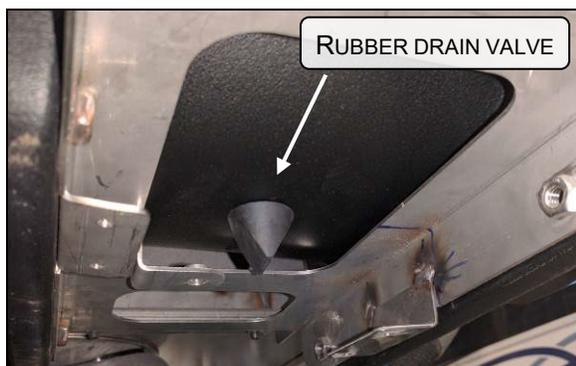
FIGURE 31 RUBBER DRAIN VALVE UNDER FILTER
