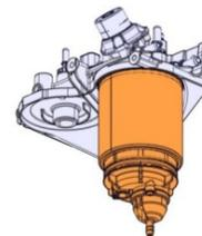
5. Unscrew and remove the water separation bowl from the filter cartridge.
