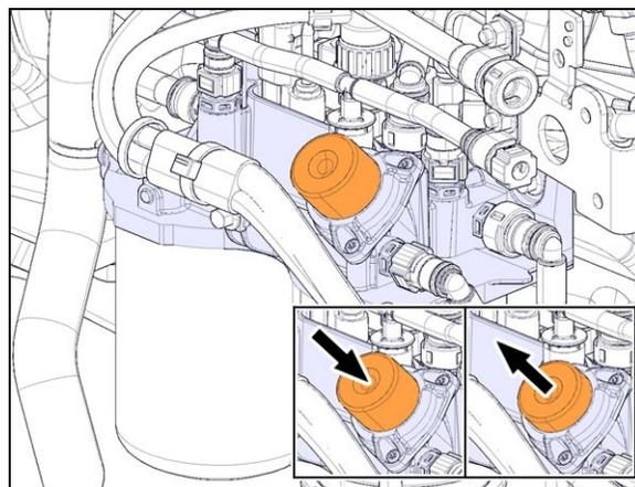
FIGURE 6: HAND PRIMING PUMP
