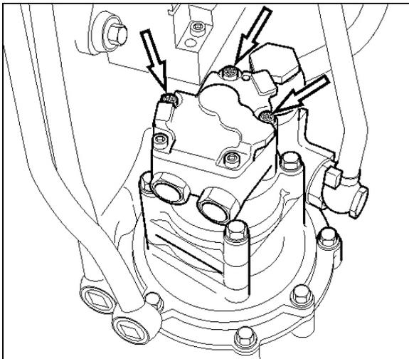
**FIGURE 12: FUEL PUMP REMOVAL**
