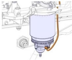
13. Open the fuel supply line shut-off valve.
