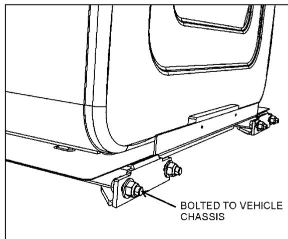
FIGURE 22: FUEL TANK SUPPORT MOUNTING BOLTS
