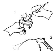
7. Check that the drainage hole in the water separator bowl is not blocked.
