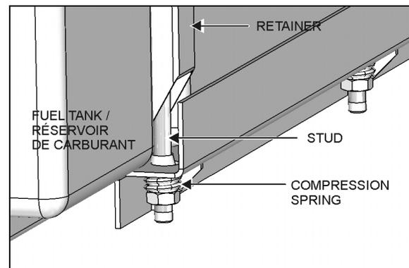
FIGURE 16: FUEL TANK RETENTION 03019\_2
