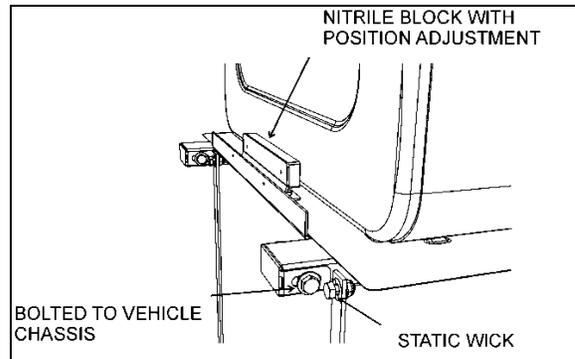
FIGURE 21: FUEL TANK SUPPORT MOUNTING BOLTS
