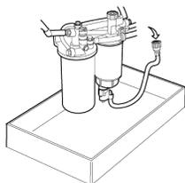
4. Unscrew and remove the primary fuel filter assembly from the fuel filter housing. Drain filter.
