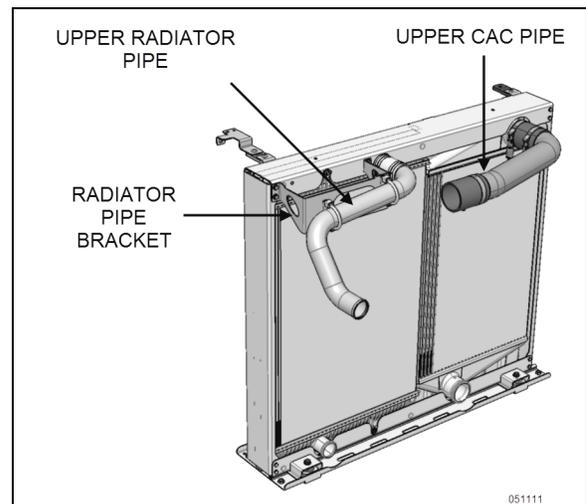
FIGURE 57: INSTALLED RADIATOR & CAC UPPER PIPES
