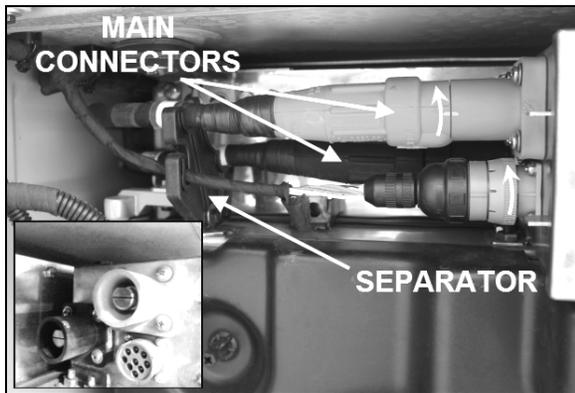
FIGURE 24: CIRCUIT BREAKER BOX CONNECTIONS
