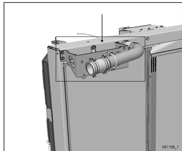
**FIGURE 41: INSTALLED RADIATOR UPPER PIPE & BRACKET**
