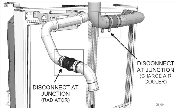
FIGURE 45: RADIATOR & CAC UPPER CONNECTION
