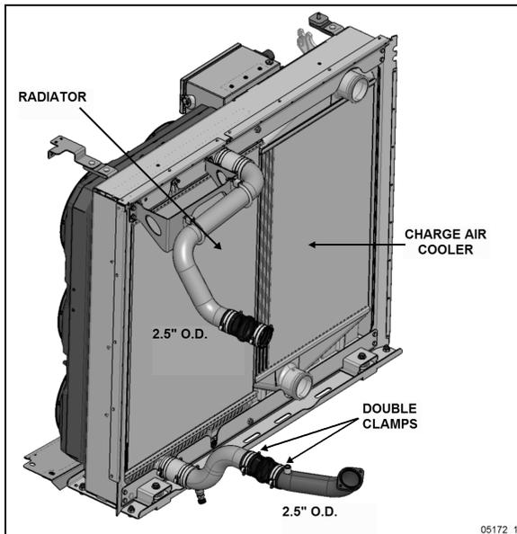
FIGURE 11: COOLANT FLOW (X3 SERIES SHOWN)
