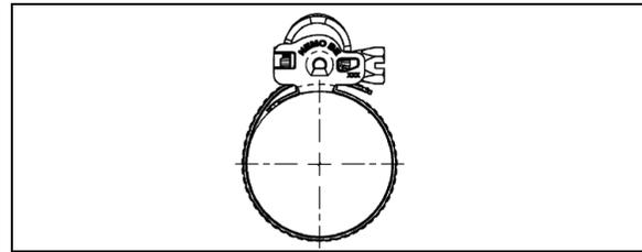
FIGURE 12: CLAMP TYPE USED ON HEATING & COOLING SYSTEMS
