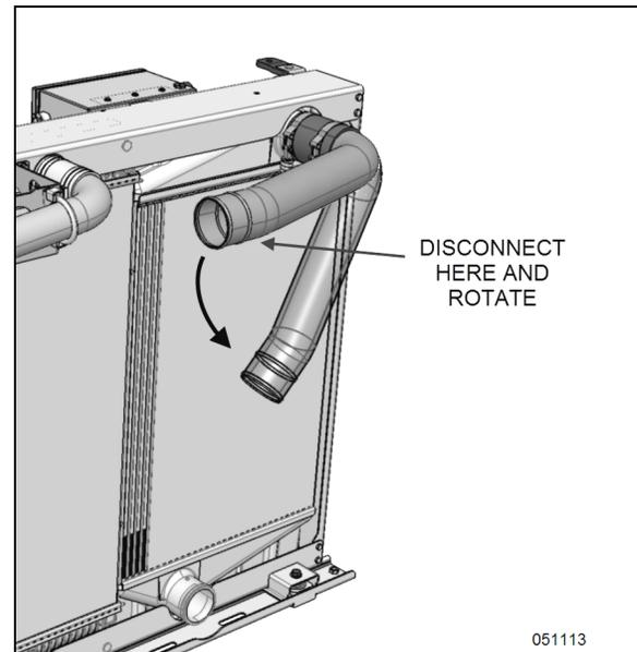
FIGURE 58: ROTATE CAC UPPER PIPE (X3 SERIES ONLY)
