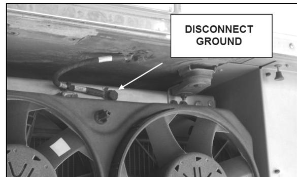
FIGURE 32: COOLING ASSEMBLY GROUND
