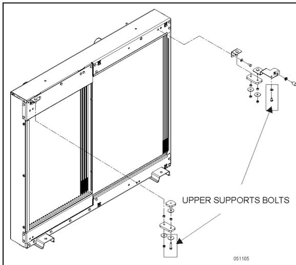
FIGURE 36: UPPER SUPPORTS MOUNTING BOLTS
