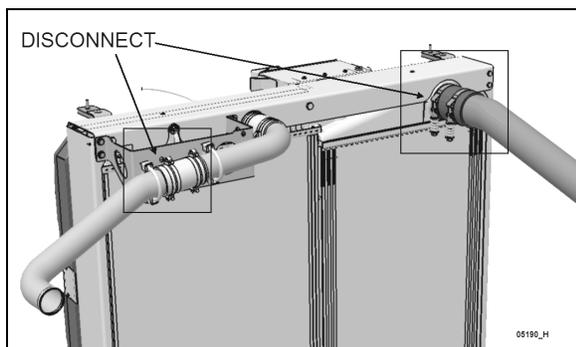
FIGURE 30: RADIATOR & CAC UPPER CONNECTION
