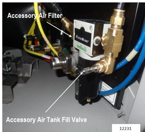
FIGURE 4: FRONT SERVICE COMPARTMENT
