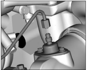
FIGURE 14: AFTERTREATMENT HYDROCARBON DOSER
