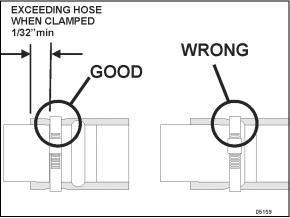
FIGURE 13: PROPER HOSE CLAMP INSTALLATION
