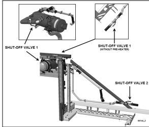
FIGURE 28: HEATER SHUT-OFF VALVES POSITION
