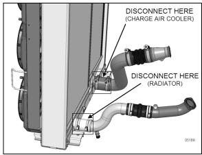
FIGURE 46: RADIATOR & CAC LOWER CONNECTION
