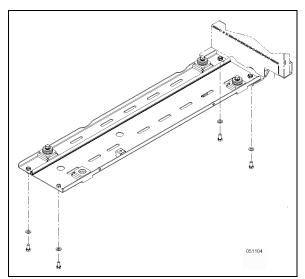
FIGURE 35: LOWER SUPPORT MOUNTING BOLTS
