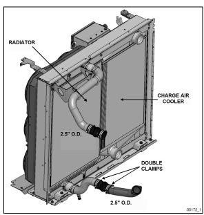
FIGURE 11: COOLANT FLOW (X3 SERIES SHOWN)
