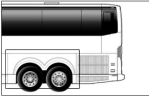
FIGURE 27: REMOVE REAR FENDER
