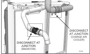
FIGURE 45: RADIATOR & CAC UPPER CONNECTION
