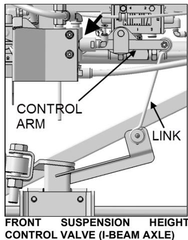
**FRONT SUSPENSION HEIGHT CONTROL VALVE (I-BEAM AXLE)**
