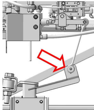
5. Loosen the lower mounting bolt shown.
