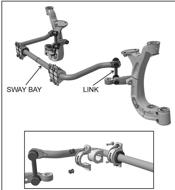
**FIGURE 34: SWAY BAR (INDEPENDENT FRONT SUSPENSION)**
