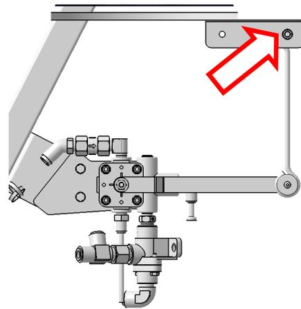
5. Loosen the lower mounting bolt shown.
