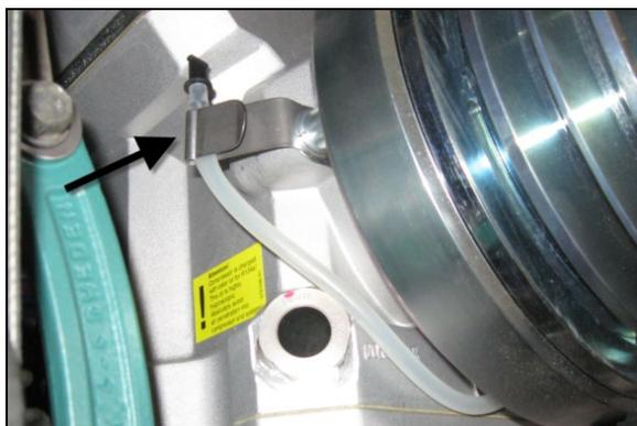
FIGURE 44: SHAFT SEAL OIL COLLECTING TUBE
