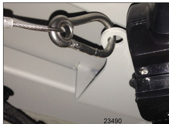
FIGURE 12: PROTECTIVE WIRE INSTALLATION
