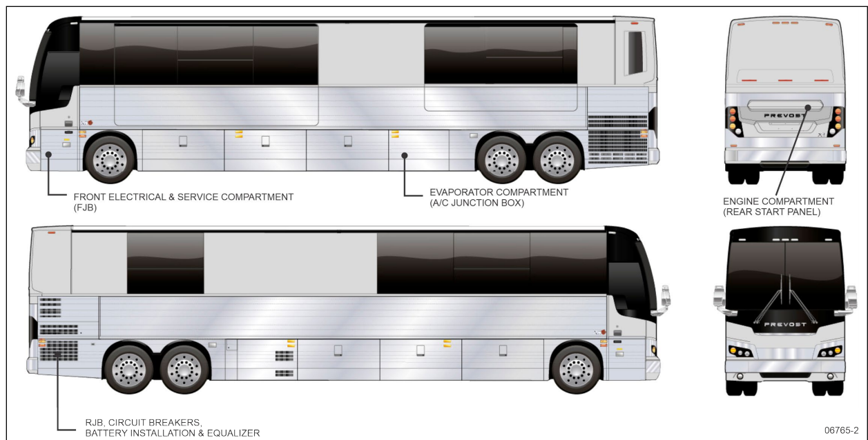
FIGURE 19: ELECTRICAL COMPARTMENTS (X3-45 VIP)
