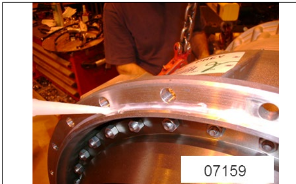
FIGURE 12: SILICONE APPLICATION TRANSMISSION HOUSING
