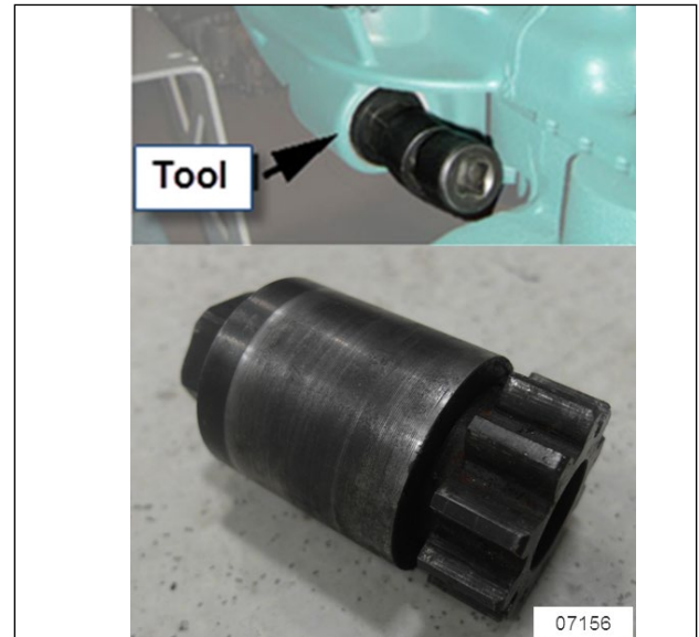
FIGURE 10: VOLVO ENGINE TURNING TOOL #88800014
