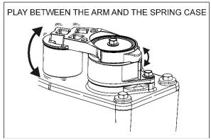
FIGURE 26: CHECKING BUSHING WEAR
