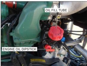
FIGURE 12: TYPICAL ENGINE OIL FILLING TUBE
