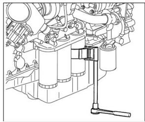
FIGURE 10: OIL FILTER WRENCH
