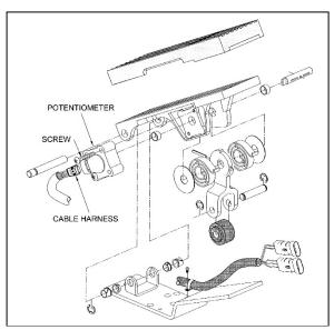
FIGURE 18: ELECTRONIC FOOT PEDAL ASSEMBLY 3035
