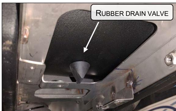
FIGURE 44 RUBBER DRAIN VALVE UNDER FILTER
