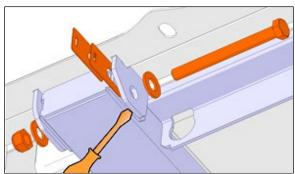
FIGURE 42: SHIM INSTALLATION, TRANSVERSE SCREW. ARRANGEMENT MAY VARY
