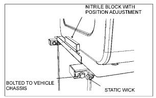
FIGURE 34: FUEL TANK SUPPORT MOUNTING BOLTS
