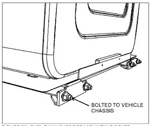
FIGURE 35: FUEL TANK SUPPORT MOUNTING BOLTS
