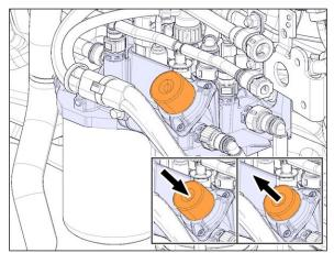
FIGURE 19: HAND PRIMING PUMP
