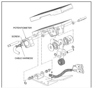
FIGURE 50: ELECTRONIC FOOT PEDAL ASSEMBLY 03035
