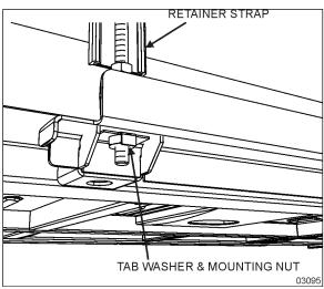
FIGURE 36: FUEL TANK STRAP MOUNTING
