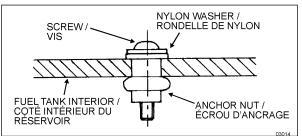
FIGURE 30: FUEL TANK REPAIR
