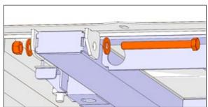
FIGURE 39: TRANSVERSE SCREWS, 2 LOCATIONS
