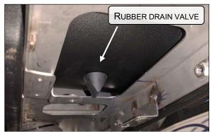
FIGURE 44 RUBBER DRAIN VALVE UNDER FILTER
