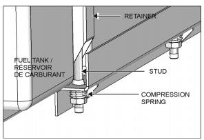
FIGURE 29: FUEL TANK RETENTION 03019\_
