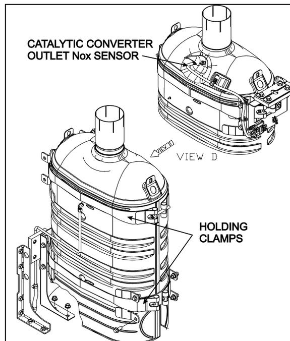
FIGURE 6: CATALYTIC CONVERTER
