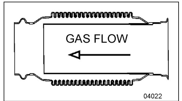
FIGURE 2: FLEXIBLE COUPLING
