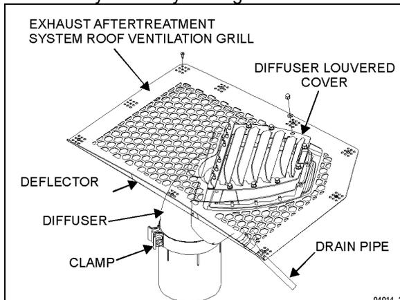
FIGURE 7: DIFFUSER ASSEMBLY
