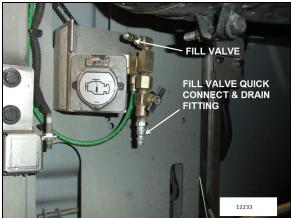
FIGURE 12: REAR VALVE LOCATION (TYPICAL)
