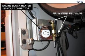
FIGURE 44: REAR VALVE LOCATION ON H3 SERIES
