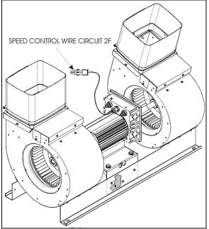
FIGURE 57: EVAPORATOR MOTOR ASSEMBLY
