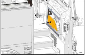
FIGURE 105:REMOVE FRONT A/C COVER TO ACCESS MODULES
