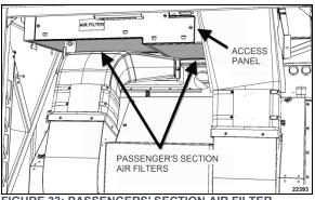
FIGURE 33: PASSENGERS' SECTION AIR FILTER
