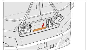
FIGURE 27: DRIVER HVAC SYSTEM FRESH AIR FILTER Two <u>recirculating air</u> filters are located under the central utility compartment.
