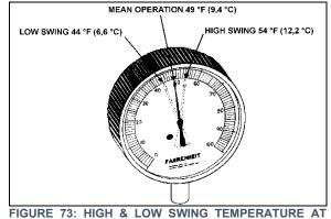
FIGURE 73: HIGH & LOW SWING TEMPERATURE AT REMOTE BULB 22047
