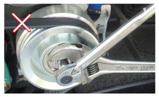
8) Once properly tighten, apply a torque seal mark.
