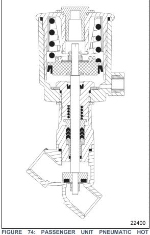
WATER VALVE - TYPICAL CUT-OUT VIEW
