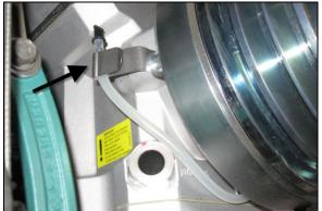
FIGURE 44: SHAFT SEAL OIL COLLECTING TUBE
