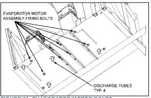
FIGURE 56: EVAPORATOR MOTOR BOLTS 22315
