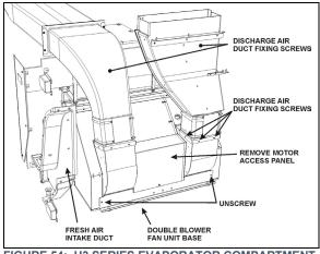
FIGURE 54: H3 SERIES EVAPORATOR COMPARTMENT
