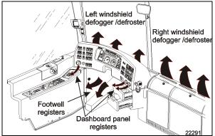
FIGURE 102: DRIVER UNIT AIR CIRCULATION
