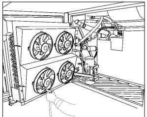
FIGURE 24: CLEANING PASSENGER UNIT CONDENSER COIL WITH LOW-PRESSURE AIR JET 22362
