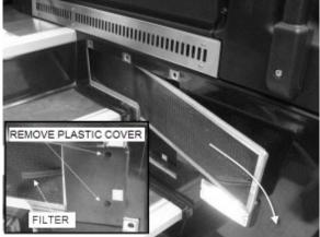
FIGURE 26: REMOVING DRIVER'S SECTION AIR FILTERS
