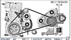
FIGURE 40: BELT LAYOUT WITH SMALL A/C COMPRESSOR H-SERIES
