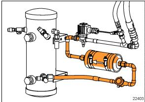
FIGURE 64: ISOLATED SECTION X3 SERIES
