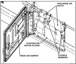
FIGURE 55: X3 SERIES EVAPORATOR COMPARTMENT
