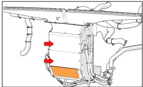
FIGURE 22: DRIVER UNIT CORE ACCESS - H3 SERIES
