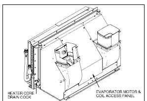
FIGURE 30: PASSENGER UNIT EVAPORATOR COIL 22332
