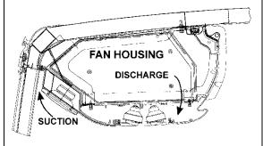
FIGURE 84: OVERHEAD COMPARTMENT VENTILATION SYSTEM 22211
