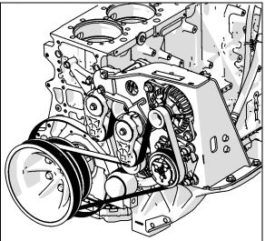
FIGURE 100 X3 SERIES SMALL A/C COMPRESSOR
