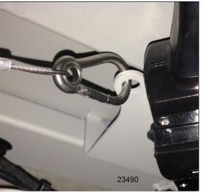
FIGURE 45: PROTECTIVE WIRE INSTALLATION
