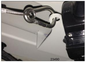
FIGURE 47: PROTECTIVE WIRE INSTALLATION
