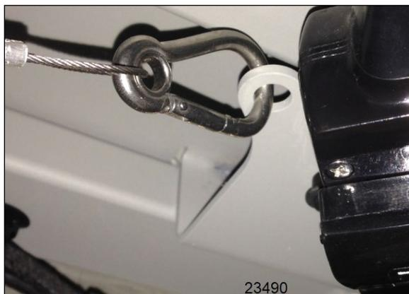
FIGURE 47: PROTECTIVE WIRE INSTALLATION
