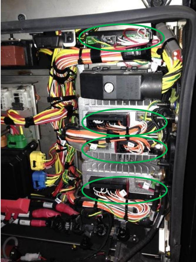
6 Disconnect the control connector from the battery equalizer
