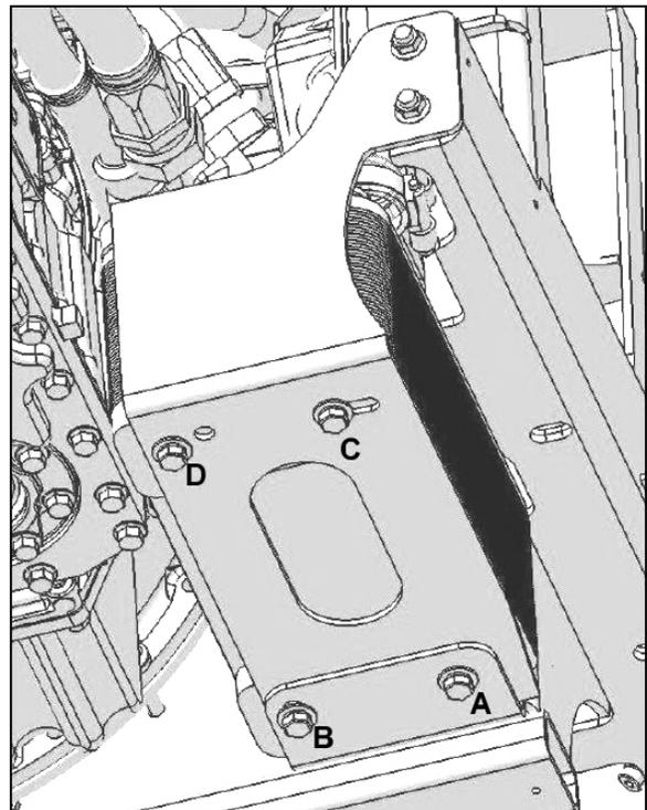
FIGURE 14: COOLER POSITION DURING ENGINE CRADLE INSERTION OR REMOVAL
