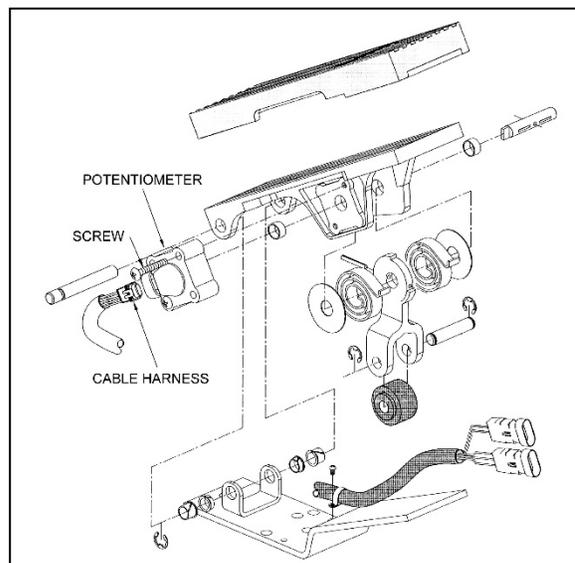
FIGURE 18: ELECTRONIC FOOT PEDAL ASSEMBLY 3035
