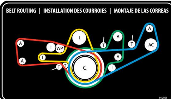
FIGURE 21: VIP BELT ROUTING – SMALL A/C SYSTEM, 5 ALTERNATORS
