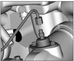
FIGURE 14: AFTERTREATMENT HYDROCARBON DOSER
