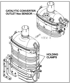
FIGURE 6: CATALYTIC CONVERTER
