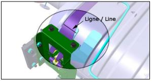
Before tightening the parts, make sure that the catalytic converter lower support is well
