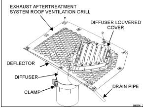
FIGURE 7: DIFFUSER ASSEMBLY
