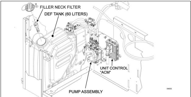
FIGURE 12 X SERIES DEF TANK AND PUMP
