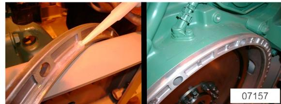
FIGURE 11: SPACER INSTALLATION
