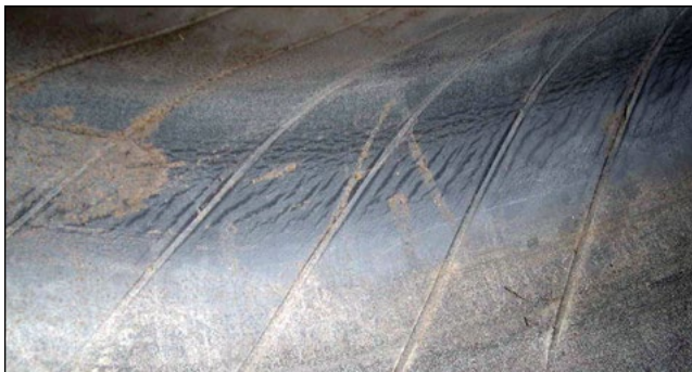
EFFECT: Inner Liner Marbling - Creasing CAUSE: Underinflation
