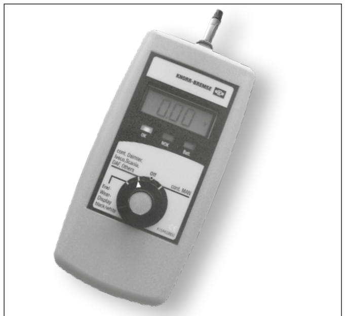
5.1.13 - Knorr-Bremse diagnostic unit K154433N50
