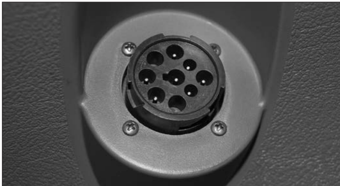
FIGURE 14 - TYPICAL VEHICLE DIAGNOSTIC CONNECTOR LOCATIONS (J1939)
