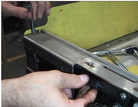
FIGURE 4-13: ROLSTOP ADJUSTMENT TOOL (GAUGE)
