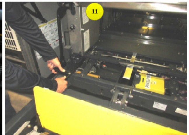
Engage lift by engaging the manual release handle, turn clockwise, and push lift in slightly. Install top cover, and cycle lift 3 times min, to check for proper operation. Check lift against stow lock and make sure it breaks away.
