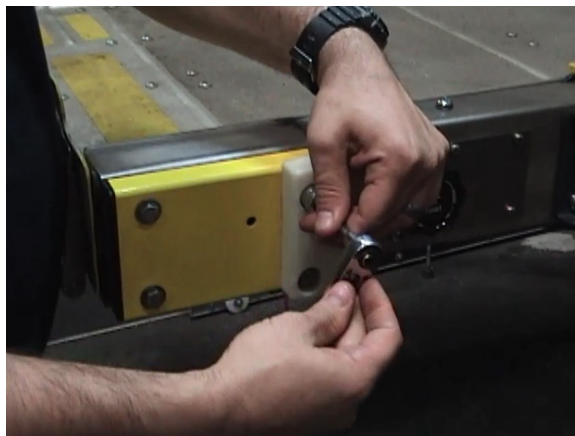
FIGURE 4-8: REMOVE RH GUIDE BLOCK AND RH PLATFORM ROLLSTOP SWITCH COVER
