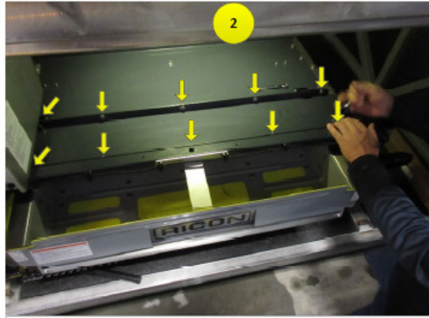
Remove the 10 pcs of 7/16" bolts holding the cover on top of the lift
