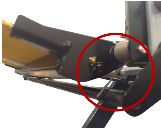
FIGURE 2-10. UNHOOK BRIDGEPLATE SPRING
