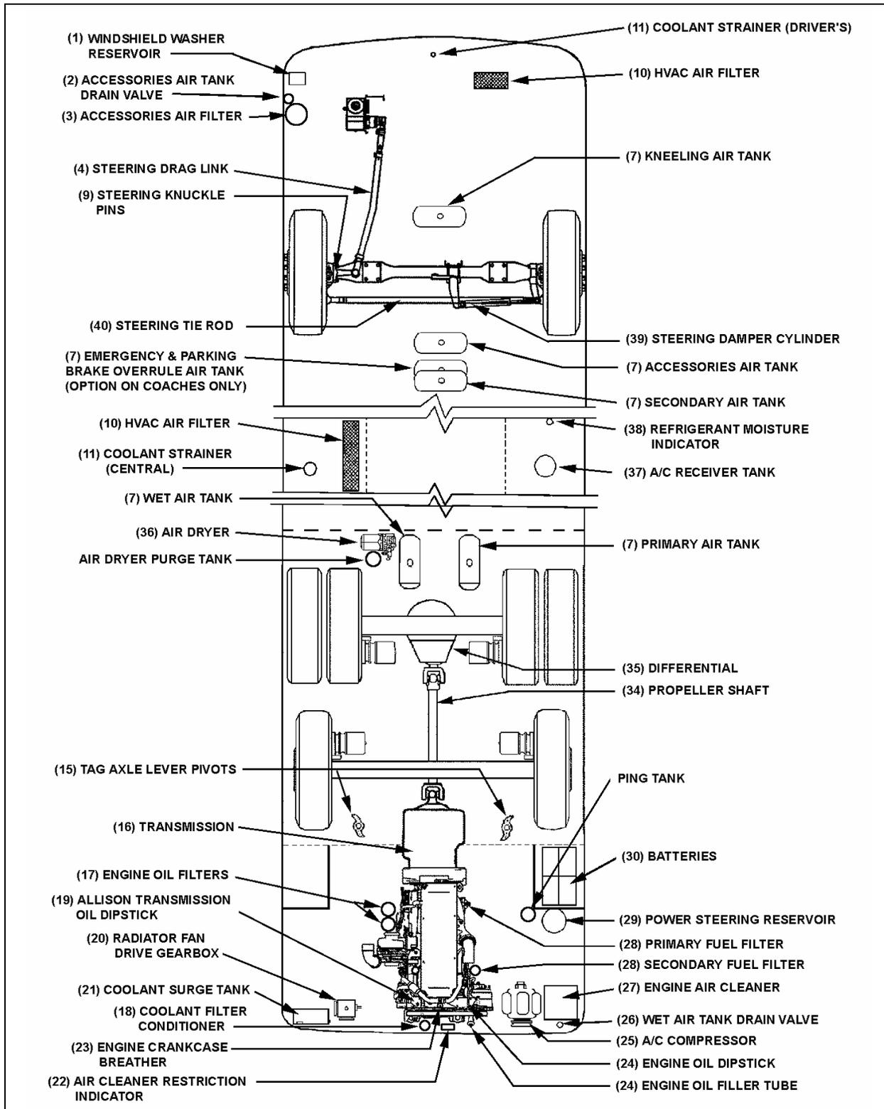
LUBRICATION AND SERVICING POINTS ON I-BEAM FRONT AXLE VEHICLES
