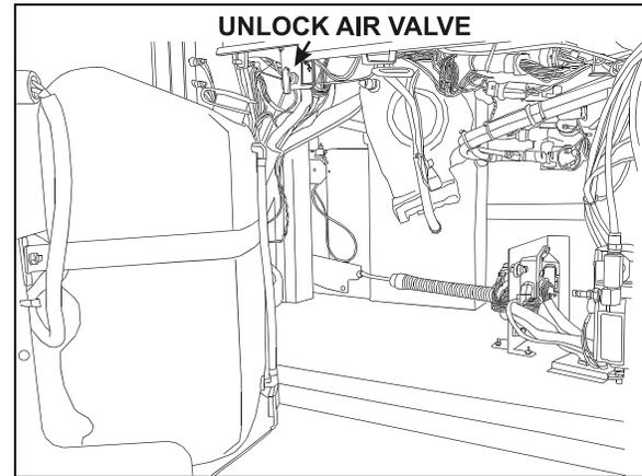
**FRONT SERVICE COMPARTMENT UNLOCK AIR VALVE**
