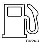
06286 Illuminates when approximately 12 US gallons (45 liters) of fuel remain in the tank. After the light comes ON, the remaining fuel will provide less than 60 miles (100 km) of travel. Do not exceed this distance. Refuel as soon as possible.
