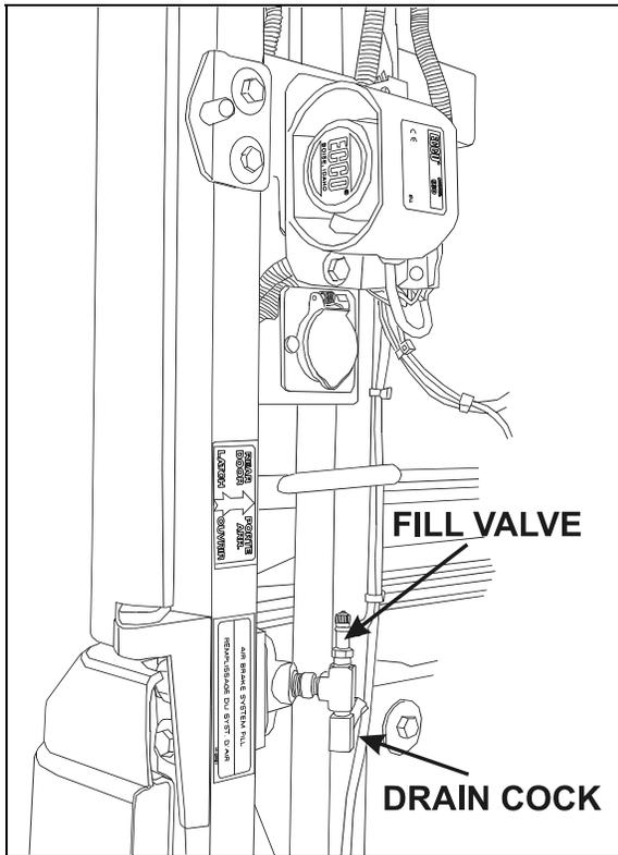
**FILL VALVE IN ENGINE COMPARTMENT** 12201
