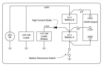
The system must be wired as shown to prevent Reverse Polarity Damage to polarity sensitive12 volt loads while the ground-side disconnect switch is open. The *VANN-Guards* GND terminal <u>must</u> be wired to the battery side of the ground-side disconnect switch circuit for the *VANN-Guard* to work properly.
