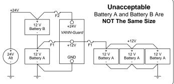
In certain applications, such as private coach or alternate energy applications, it may be desirable to have additional 12 volt "House Batteries" to operate heavy 12 volt (inverter) loads. Use the *VANN-Guard* to charge the additional batteries.
