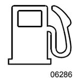
Illuminates when approximately 12 US gallons (45 liters) of fuel remain in the tank. After the light comes ON, the remaining fuel will provide less than 60 miles (100 km) of travel. Do not exceed this distance.
