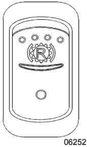
Press down this rocker switch to activate the transmission retarder.
