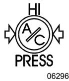
Illuminates when the A/C system pressure is too high. If the A/C pressure is too high, the compressor clutch is disengaged, but the fan remains activated.
