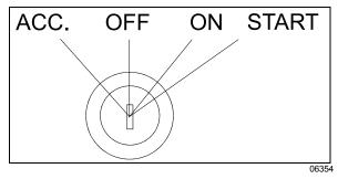
The ignition switch is located on the lower left side of the dashboard. It has four positions:
