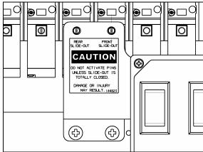
LOCKING PIN VALVE PROTECTION PLATE
