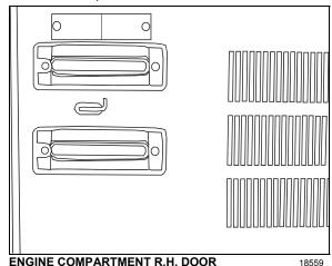
This door can be locked or unlocked using the exterior compartment key or, if so equipped, by the central door locking system. To open, push sideways the small lever located between the marker lights.
