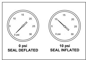
**INFLATABLE SEAL PRESSURE GAGE**
