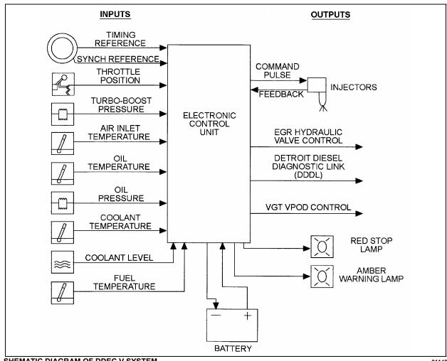
SHEMATIC DIAGRAM OF DDEC V SYSTEM
