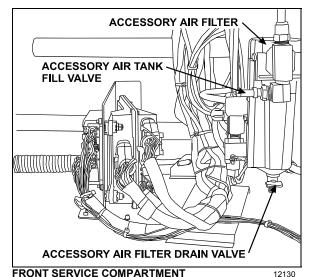
Both air system emergency fill valves are fitted with standard tire valve stems. The air systems can be filled using any standard external air supply line. The fill valve located in the engine compartment supplies air for all systems (brakes, suspension and accessories). The fill valve located in the service compartment supplies air for accessories only.
