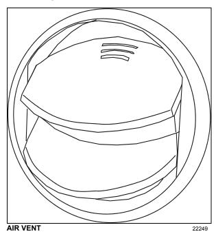
Three adjustable driver air vents in the dashboard and one near the door feed air to the driver's compartment. Use the HVAC control panel to set air temperature.
