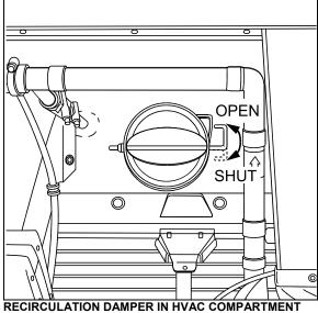
Open or close the recirculation damper with the lever shown in the illustration above
