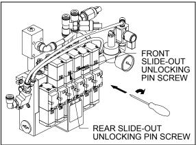
UNLOCKING PIN VALVE LOCATION
