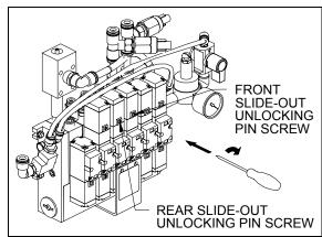
UNLOCKING PIN VALVE LOCATION
