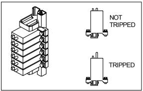
**BREAKERS IN SLIDE-OUT CONTROL COMPARTMENT**
