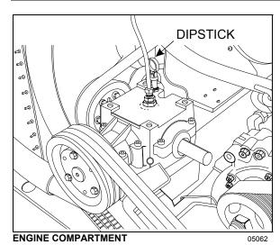
Add, if necessary, MOBIL SHC 630 synthetic lubricant (Prévost #180217) until it reaches "FULL" mark;
