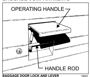
The baggage compartment doors of the XL2-45 model provide 407 ft³ (11,53 m³) of storage space (the XL2-40 has 315 ft³ [8,9 m³] of storage capacity). The compartments can be locked or unlocked by using the exterior compartment key. Pull up operating handle to release the latch, and then pull the door open. Pressurized cylinders assist the opening and closing of the baggage compartment doors and hold the doors open.
