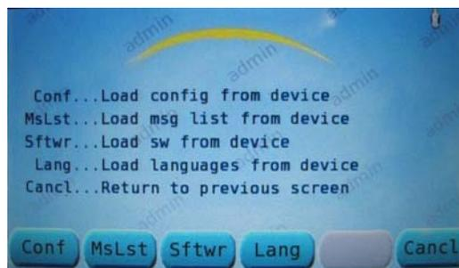
**Figure 7-22. Load From Device Menu**
