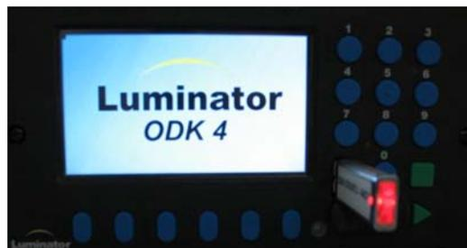
Figure 7-1. Flashdrive Inserted into ODK4
