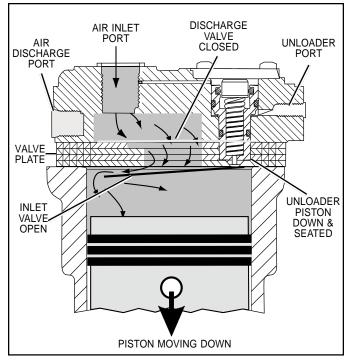
FIGURE 4 - OPERATIONAL-LOADED (INTAKE)
