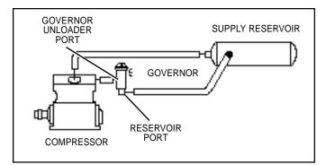
FIGURE 3 - BA-921 COMPRESSOR UNLOADER SYSTEM
