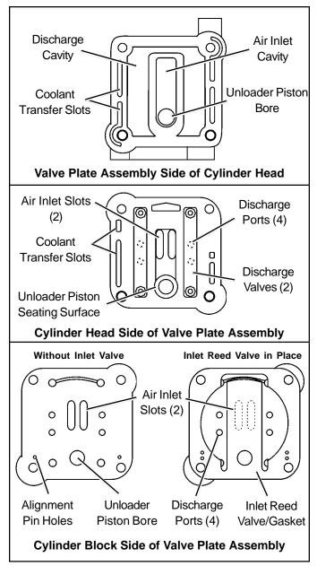
FIGURE 7 - CYLINDER HEAD AND VALVE PLATE ASSY.
