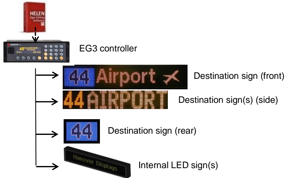
Figure 1 - diagram showing typical controller / signs configuration. Each unit is powered individually.
