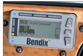
Example of Driver Interface Unit (DIU) detected forward vehicle display
