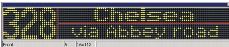
Template for sign with three areas; Line number, destination, and Via destination
