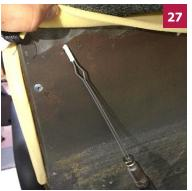
Push in the foam on the front and retract the pull tab through the steel back panel hole and rotate 90°. Repeat for all three pull tabs.
