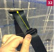
Reinsert the belt guide into the upholstery opening so that the upper tab is behind the upholstery.
