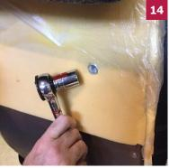
Remove the belt housing bolt with a 17 mm socket wrench.
