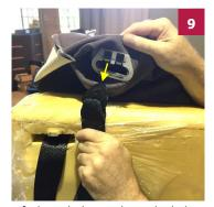
Lift the upholstery above the belt guide area and slide the belt end through the belt retainer (from the outside to the inside of the upholstery).
