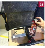
Pull the upholstery down to the armrest level and add spray glue on the lower portion of the back panel.
