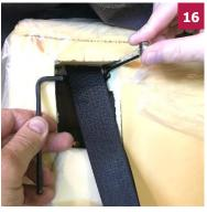
Through the front opening loosen the belt roller guide with a 3/16" hex (Allen) and a 7/16" open end wrench.
