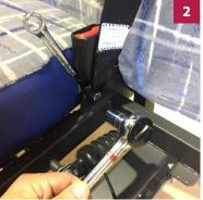
Remove belt end from the seat structure with a 5/8" socket wrench and 5/8" open end wrench.
