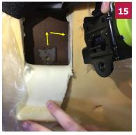
Remove belt housing retaining tab from the metal plate slot in the back by lifting, up and out.
