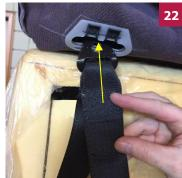
Feed the belt completely through the belt retainer (from the inside to the outside of the upholstery).
