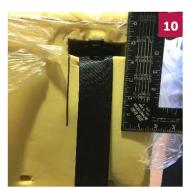
Mark two, 4" vertical lines from the bottom sides of belt openings in the foam.
