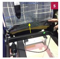
Separate the front cover *Velcro®* from Pull the upholstery up the back from the back carpet at the bottom of the the bottom, like your pulling off a back cushion upholstery.
