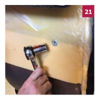
Reattach the belt housing bolt with a 17 mm socket wrench.
