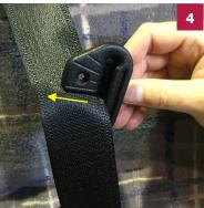
Remove the guide by bunching the belt to one side and sliding it through the vertical slot.
