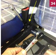
Reattached the belt end to the seat structure with a 5/8" socket wrench and 5/8" open end wrench.
