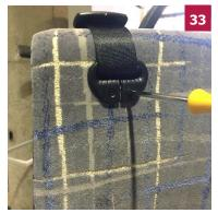
Replace belt guide screws with cross recess (Phillips) screwdriver.
