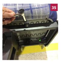
Reattach nut and washer to replace seat cushion with ½" socket wrench.
