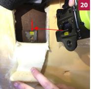
Reattach the roller guide with a 3/16" Add the new belt assembly into the opening. Hook retaining tab into the slot in the metal plate on the back. Yellow areas illustrated, face to face. Maintain vertical orientation of belt assembly so belt does not malfunction.
