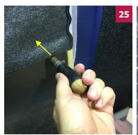
Insert a Pull Tab Tool through each opening in the back one at a time.
