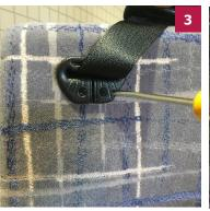
Remove two cross recess (Phillips) screws from the belt guide on the back cushion.
