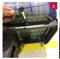
Remove nut and washer to remove seat cushion with 1/2" drive socket wrench.
