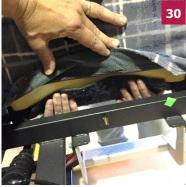
Pull back carpet down under and around bottom of the back and attach *Velcro* to carpet material.
