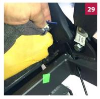
Pull the upholstery down the rest of the way and reattach *Velcro®* tabs at each corner.
