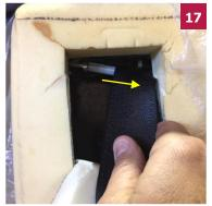
Hold onto the nut and slide the belt off the roller guide. (The belt assembly is now free from the seat.)
