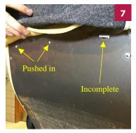
Lift upholstery and foam backer high enough to access pull tabs. Pull the tabs out, turn 90° and push into hole. Pressure on the front of the foam will create enough slack to rotate pull tabs.
