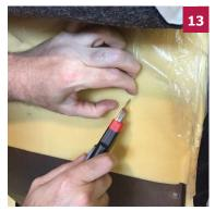
Locate the upper belt housing bolt head through the back foam and cut a small X at the location.
