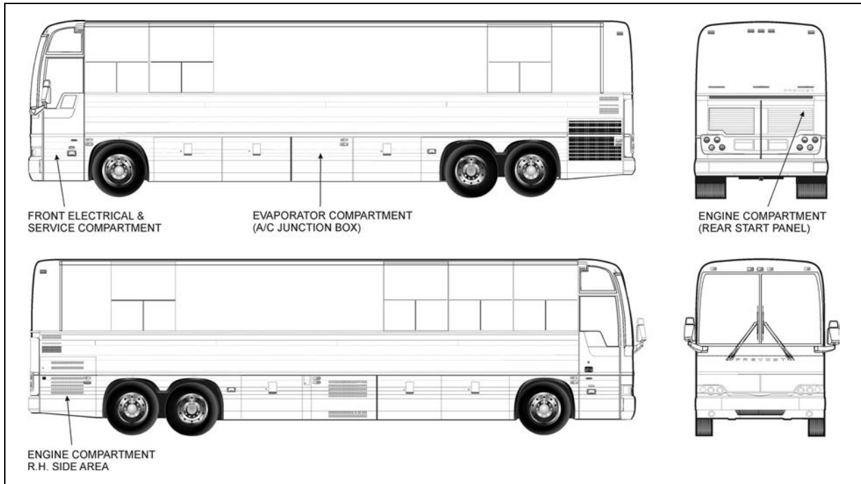
FIGURE 3: ELECTRICAL COMPARTMENTS (XLII-40 BUS SHELLS)
