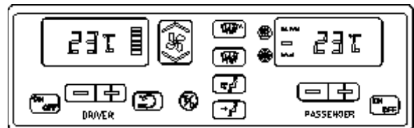
FIGURE 5: CENTRAL HVAC SYSTEM CONTROL MODULE
