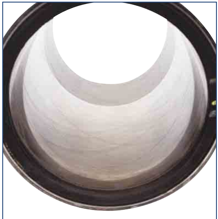
Piston liner shows cross hatch pattern intact.
