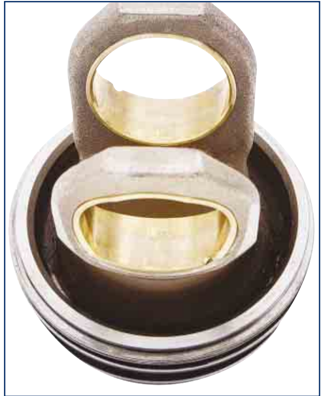
Piston bushings only show typical polishing.
